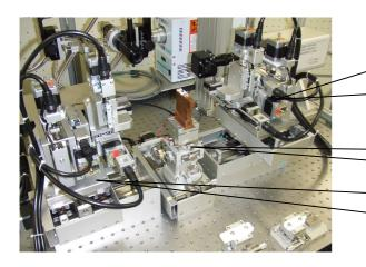
Output: Automatic Fiber array stage unit
